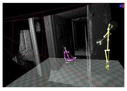
Example of the "data" provided from a sensor (fallen person marked red). SSP only uses smart sensors that fully protect personal identity – no cameras.
